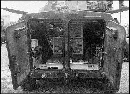
The LAV does not have a ramp; instead it has two manually operated doors.
