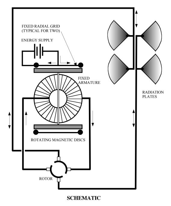
The above diagram pictures a disc arrangement where two rotating magnetic discs have a stationary armature sandwiched flat between them (not at 90 as shown in the
